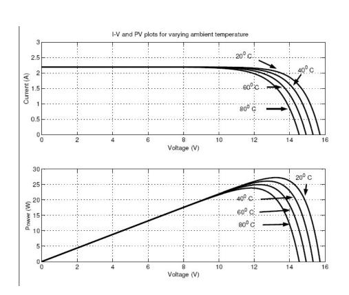
Figure 8: Temperature coefficient for crystalline cells
