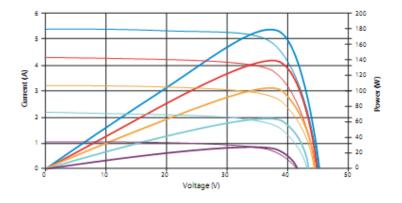
Figure 5: Maximum Power Point Tracking
