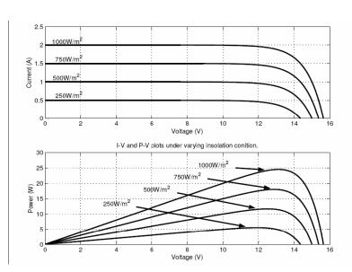
Fig. 6 Changes in the characteristics of the solar pv module due to change in insolation level
