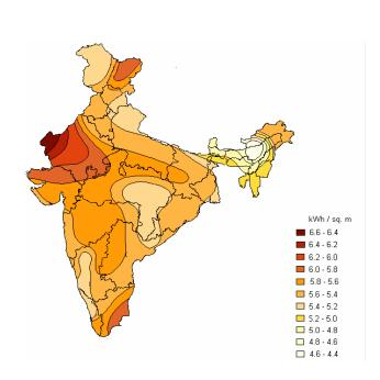
Figure.4 Solar radiation zones as per TERI based on the IMD database.
