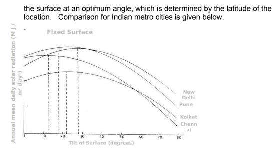
Figure 7: Global radiation at different tilt angle
