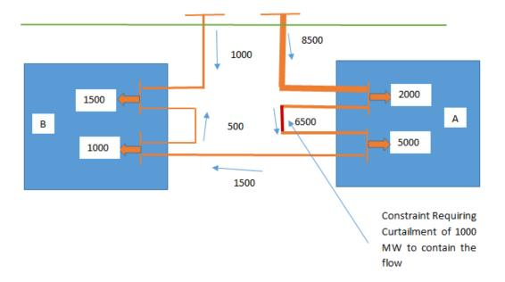
(h) To control the power flow in the congested corridor TTC as calculated by planner would need to be revised from 8500 MW to 7510 MW. Even when STU B has given correct nodal GNA its GNA gets curtailed based on the priority decided.
