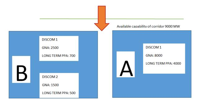
In case sum of requisitions from both the states for power import through the specific corridor exceeds the available capability due to any contingency, then the requisitions made by the States need to be rescheduled to ensure that the total requisition is equal to available capability.
