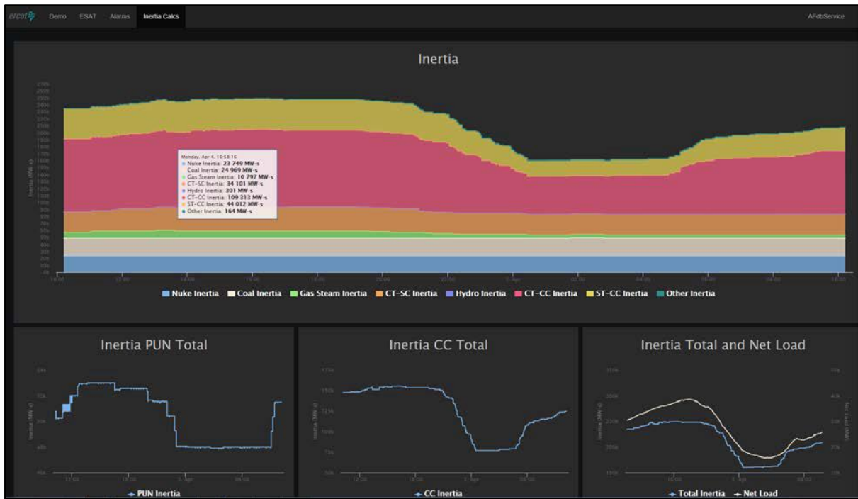
Figure 15: ERCOT dashboard to monitor the real time inertia
