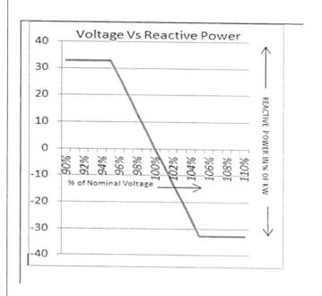
Hence reactive power injected during the period of voltage less than the nominal value and reactive power absorbed during the period of voltage more than the nominal value by any Solar/Wind Inverter based Generator, if more than the values stipulated as above, such Var exchanges in excess of the stipulated value is proposed to be compensated based on the rate of reactive power approved by CERC as stipulated in the Annexure - 4 of draft IEGC Regulation 2022.
