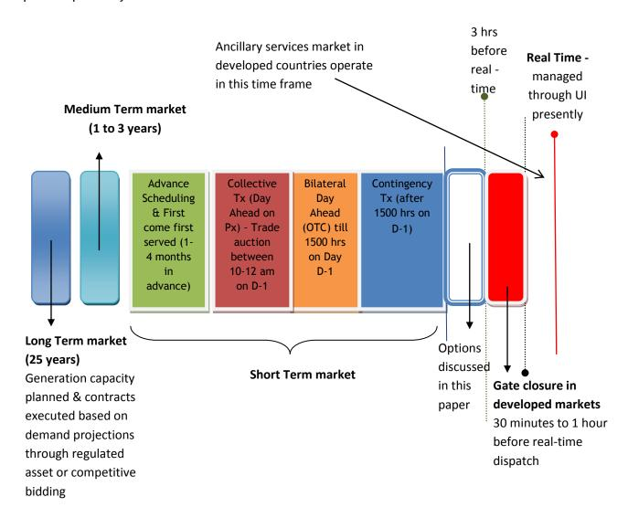
Indian market design is decentralized dispatch concept where the merit ordering and scheduling responsibility is with the Discoms and the deviation settlement mechanism provides the Automatic Generation Control (AGC) for the Indian electricity grids and the whole design encourages the gencos/utilities to conserve when in the real time balance becomes surplus and to provide for when in there is a real time shortage and thus maintaining the grid frequency.
